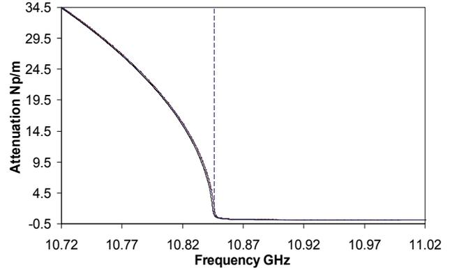
**Fig. 3.** Attenuation of TE<sub>11</sub> mode at the vicinity of cutoff. The solid line was calculated using our method, dotted line using Stratton's method, and the dashed line using the perturbation method.
