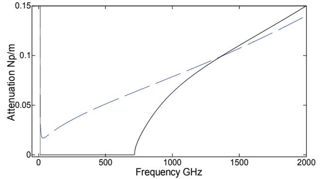
Fig. 5. Attenuation for TE<sub>11</sub> mode in a Nb circular waveguide at  $T = 4.2$  K (solid lines) and room temperature (dashed lines).
