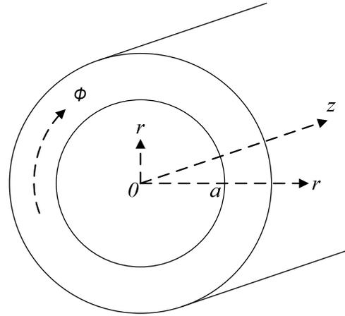
Fig. 1. A circular waveguide.
