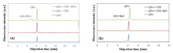
Figure 4: Electropherograms of QDs-BSA (a) and QDs-IgG (b) conjugates.
