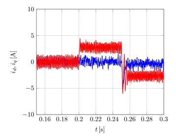
Fig. 6. Currents during load torque experiment; blue -  $i_d$ , red -  $i_q$ .
