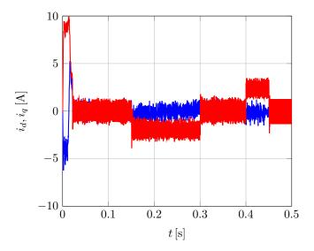
Fig. 3. Currents during reference tracking experiment; blue -  $i_d$ , red -  $i_q$ .
