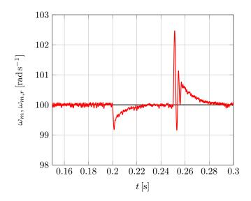
Fig. 5. Angular speed during load torque experiment; black - reference, red - measured speed
