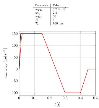
Fig. 2. Results of the reference tracking experiment; black - reference, red - measured speed.
